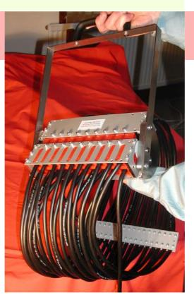
be labouriously wound and unwound at each step. This is ok for large utility pipes, but for beams in a steel structure working many metres from the ground the clam coils are the best solution.
