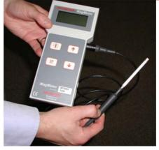
agmeter MF300H is the Diverse Gaussmeter. It is a robust field instrument that can measure magnetic field from the very low levels right up to the point where magnetic materials saturate. It is supplied with a slim but robust stainless steel probe ideal for measurement in pipe weld preps.
