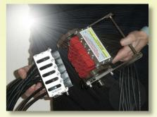
Bobbins used for pipe end degauss
