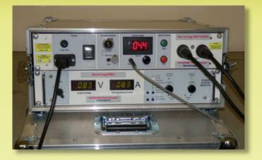
The success of demagnetising of the pipe end is dependent on the pipe material and the number of turns that can be applied. Note also that over time the magnetism in the rest of the pipe will reestablish itself in the pipe end. This occurs typically in 1-2 hours.
