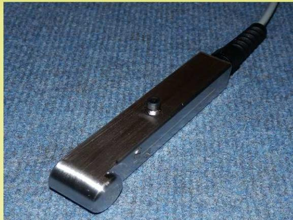
The MF500M provides an indication of the amount of magnetite within steam tubes. It assumes that the containing tube is essentially non-magnetic made usually of stainless steel. The magnetite is magnetic with magnetic properties similar to iron. This provides a route to measure the levels of
