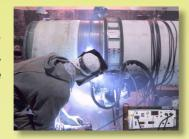
can be used on an ad hoc basis to guarantee that welding will never stop because of arc blow. However, many of our users deploy the DKPW within the production environment so that it is used for every joint. The reason is that even low levels of magnetism can cause unwanted arc wander and result in zones of porocity which will need to be ground out and rewelded. With Zeromag deployed this situation never occurs so overall production rates are increased and weld quality improves.
