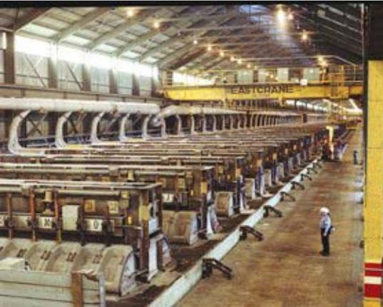
Clearly Zeromag cannot be used to combat such ferocious magnetic fields directly. However, with a combination of Zeromag ZM100A or ZM100A-30, together with suitable clam coils, the field from the smelter can be nulled and welding may proceed. Diverse use finite element analysis of the static field and the geometry of the weld set up to determine the best way to apply Zeromag.
