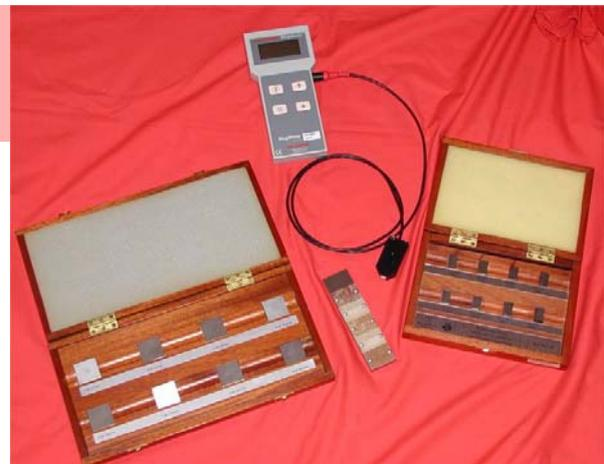
Every instrument is supplied with calibration standards that are checked with the instrument against the world standards. The MF300F reports in "ferrite number", which for many materials can be converted directly to percentage ferrite.
