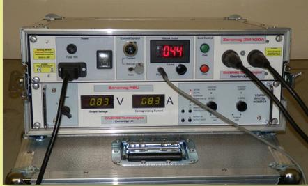
In manual mode, the user has full control over the demagnetizing current allowing accurate trimming of the magnetic field to zero. In automatic mode Zeromag takes control of the reversing current. For the user there are just 2 operating buttons: GO and STOP!
