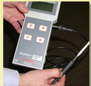
This is an ideal instrument to assess whether demagnetizing is required. Its tough slim probe can be used into the bottom of a 'V' or 'J' prep to give an accurate measurement of what field the welder will have.
