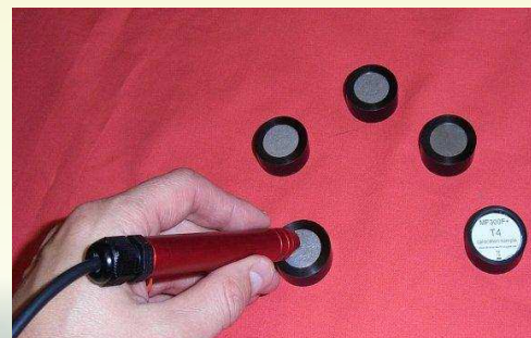
MF300F+ measuring the transfer standards
